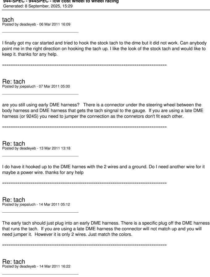
is ther any way to test the tach. i have it hooked to the original harness and nothing, the tach bounces if
